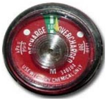
2. Check the pressure of the extinguisher. The pressure should be within the recommended level indicated on the gauge. The needle should be in the green zone. If the needle is not in green zone, the extinguisher requires professional maintenance.
